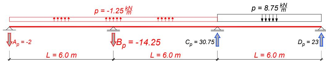
$$M_{1p} = -\left(\frac{-1.25}{15} + \frac{-1.25}{20} - \frac{8.75}{60}\right) \times 6.0^2 = 10.5 \text{ kNm} \Rightarrow A_p = \frac{-1.25 \times 6.0}{2} + \frac{10.5}{6.0} = -2.0 \text{ kN}$$
