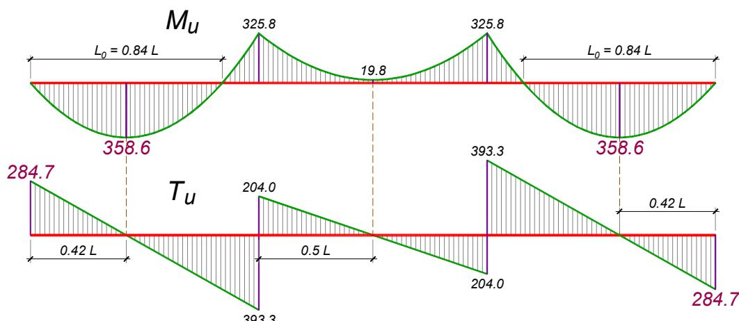
$$L_0^{01} = 2x_{\max} = 2 \times 2.52 = 5.04 \text{ m} \Rightarrow B = \min \left\{ \begin{array}{l} 40 + 20 \times 14 = 320 \\ 40 + 0.25 \times 504 = 166 \end{array} \right\} = 166 \text{ cm}$$
