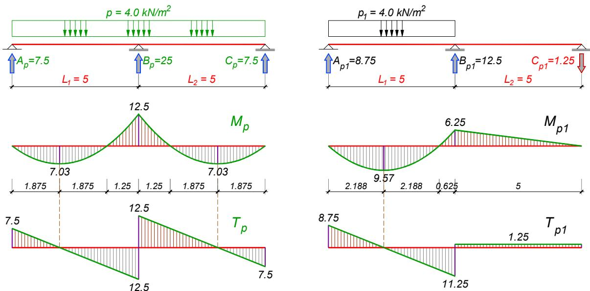
$$A_{u,\max} = 1.6 \times A_g + 1.8 \times A_{p1} = 1.6 \times 11.25 + 1.8 \times 8.75 = 33.8 \frac{kN}{m}$$
