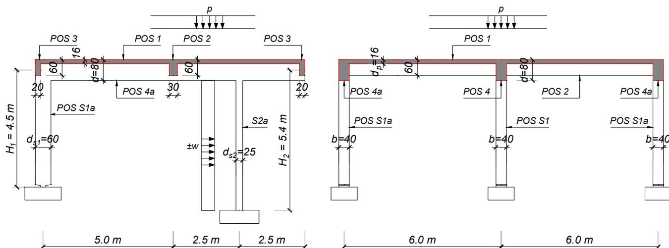
$p = 8 \text{ kN/m}^2$      $w = \pm 20 \text{ kN/m}^1$     MB 30    RA 400/500
