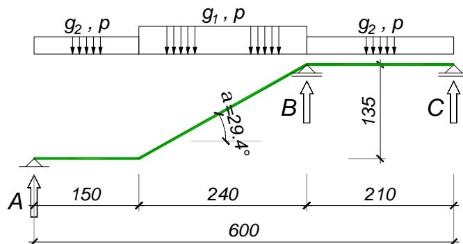
$$d_p \geq \frac{L_0}{30} \approx \frac{0.8 \times 390}{30} = 10.4 \text{ cm} \quad \Rightarrow \quad \text{usvojeno } d_p = 14 \text{ cm}$$
