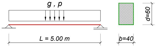
$$\left. \begin{array}{l} M_g = 24 \times 5.0^2 / 8 = 75 \text{ kNm} \\ M_p = 32 \times 5.0^2 / 8 = 100 \text{ kNm} \end{array} \right\} \Rightarrow M_u = 1.6 \times 75 + 1.8 \times 100 = 300 \text{ kNm}$$
